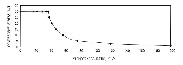
Figure 11-1. Typical column strength curve
